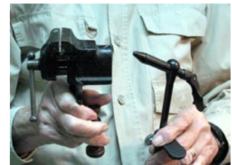
A small vise and a fly tying vise are among the tools you'll find lots of use for in your down time tackle repair and preparation. I'm forever using one or the other for a variety of purposes.
